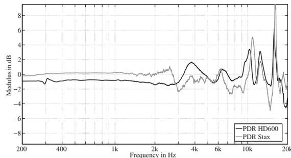
**Figure 8:** Pressure division ratio for headphones Stax SR Lambda and Sennheiser HD600. Average of eight HpTF measurements made with the help of a mounting device to reduce high frequency variability and HRTF measured for five different directions.
